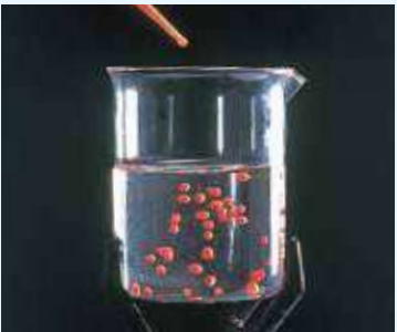
Example : spherical gel particle production : spiking drops of a 1% aqueous alginate solution with orange colorant into a 1% calcium chloride aqueous solution.
